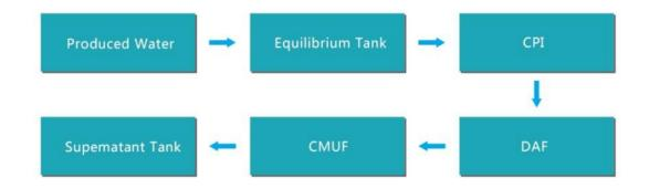
The oil contained wastewater firstly passes through the equilibrium tank skimmer unit to adjust flow rate and remove slick oil; then in the DAF unit emulsified oil will be largely reduced; finally through the CMUF unit, most of SS and oil content of wastewater will be cleaned up to meet the  $0.01\mu$  m2 average air permeability standard of SY/T5329-2012.
